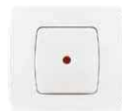
Jednopolna sklopka sa signalnom sijalicom i nulom Single-pole switch with pilot light and zero contact 16AX/250V; IP 20
